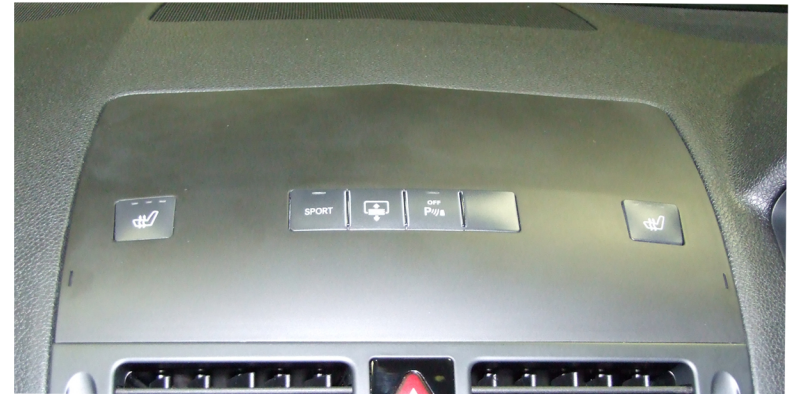
Install New Relocation Panel . The panel is very tight to clip in place, you will need to clip the top hooks first then lower clips.
