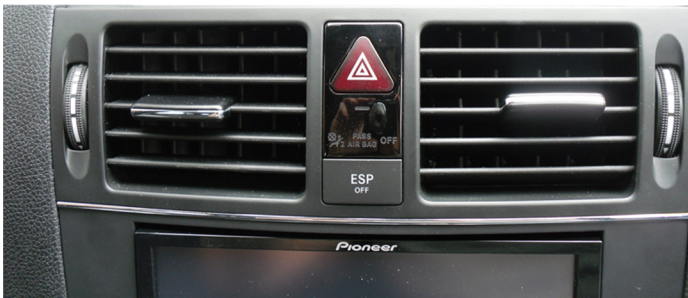
Slide airvent panel back into the place.
